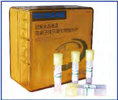
Biological indicator(self-contained) Bacteria: Thermophilic fat bacillus Quantum: 2-5*10 6
